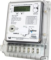
**VTX-34G** is Electronic Three Phase Four Wire Whole Current GSM/GPRS Energy Meter developed for residential and commercial users. This meter is developed for measurement of Active and Re-active energy and also includes maximum demand and Multi-tariff features. This model upholds advanced Anti- Tempering features and suitable for high power theft areas. current.
