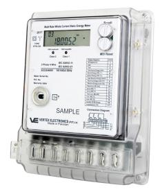
VTX-34 is Electronic Three Phase Four Wire Whole Current Energy Meter developed for residential and commercial users. This meter is developed for measurement of Active and Re-active energy and also includes maximum demand and Multi-tariff features. This model upholds advanced Anti- Tempering features and suitable
