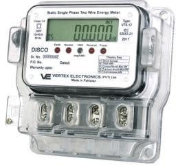
**VTX-12** is Electronic Single Phase Two Wire Energy Meter mainly developed for domestic and commercial applications. This model upholds comprehensive Anti-Tempering features and suitable for high power theft areas. Meter is capable to record energy even when neutral is missing or in case of reverse current.
